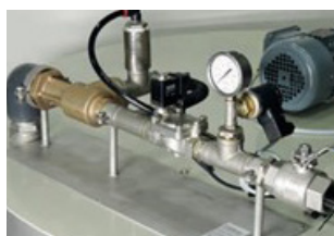
Inlet armatures including the high-effective injection nozzle.
